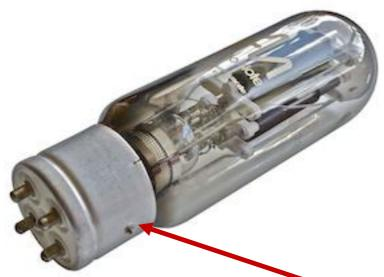
Inspect a 211 valve and you will notice that there is a small 'pin' protruding from one side of the valve base; this locating pin ensures that the valve can only be correctly inserted into the amplifier in one way.
