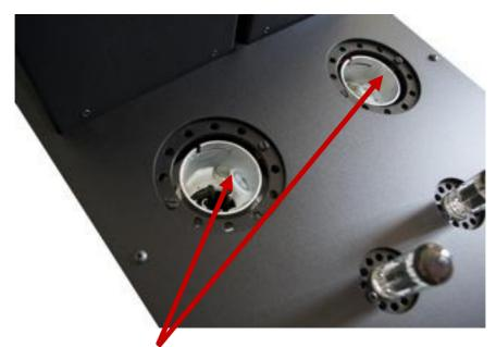
Also examine the two large apertures in the top plate of the amplifier, located between the two small valves and the black rectangular transformer covers. These are the insertion points for the 211 valves.
