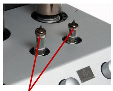
Finally, insert the two small signal valves into the front two sockets. Looking from the front of the amplifier, insert the taller 7044 valve into the left socket, and the smaller ECC82 into the right socket. The valves can only be inserted one way.
