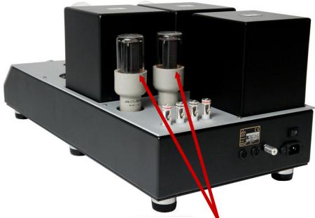
Looking from the back of the amplifier, insert the **5R4WGB** valves into the two empty sockets located on the left, situated between the black rectangular transformer covers and the loudspeaker connection binding posts. Locate the rib on the central pin of the valve and align with the valve base (it can only be inserted one way due to this locating rib) and with gentle but firm pressure insert the valve.
